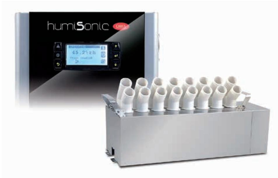
Installed directly in the air flow, humiSonic ventilation makes adiabatic humidification available also in smaller ducts, offering a high energy efficiency alternative to steam humidification. Power consumption per kg of evaporated water is in fact less than 80 W, around 90% lower.
